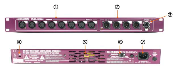
Input sockets 8 balanced XLR inputs for microphone and line level sources. The preamps are built into the AR84 rack and their Gain, Pad and 48V phantom power is remote controlled from the mixer via the digital link. The output of the analogue preamps are converted to digital format and transported via a Cat5 cable to be processed and mixed at the GLD or Qu mixer.
