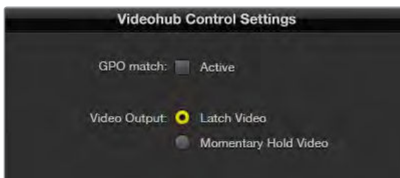
Select Latch Video if you want your preview to hold until another crosspoint is selected. Choose Momentary Hold Video if you want your preview to revert back to the previous crosspoint when you release the control switch.
