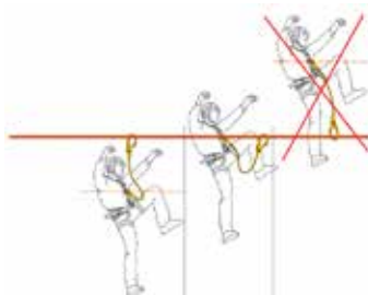
Fall arrest system with shock absorber
