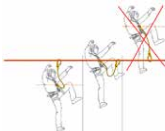
Fall arrest system with shock absorber
