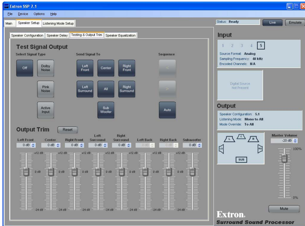
Figure 23. Testing & Output Trim Tab
