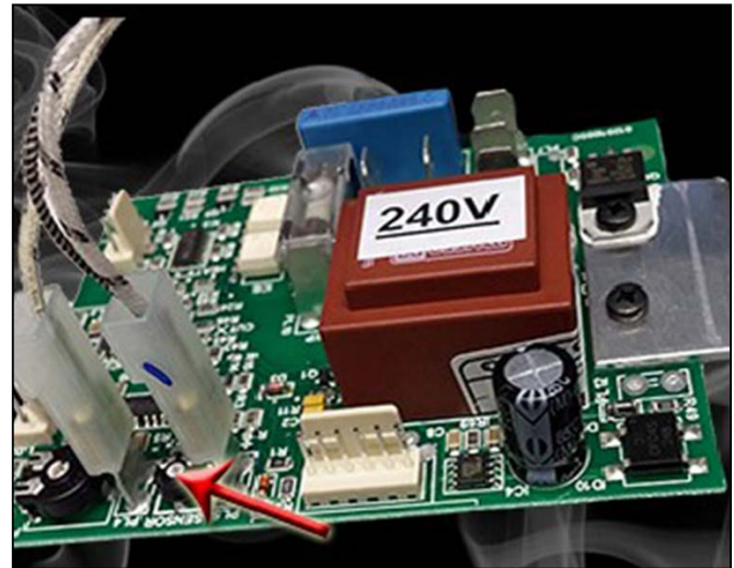
Figure 21: Disconnecting thermocouple wires
