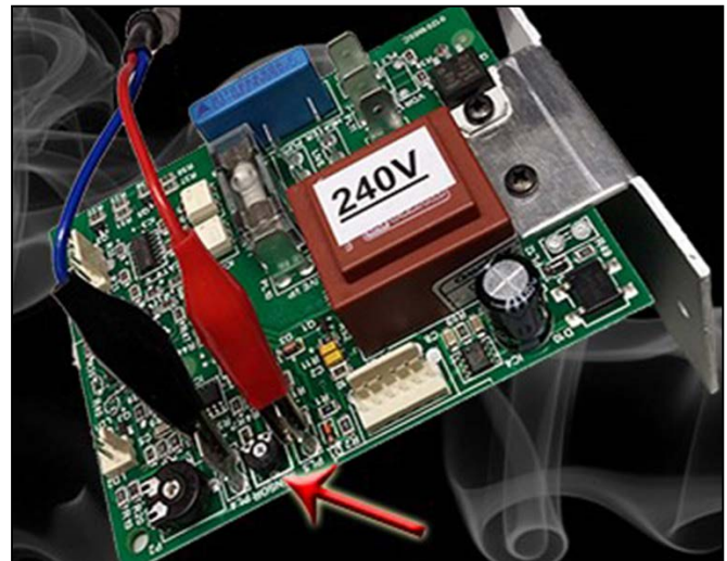
Figure 22: Replacing thermocouple wires
