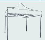
Adjust the height of the tent using the extendable legs. To do this, push the pin on the leg inwards
