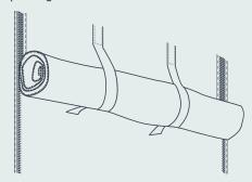
Unzip the two vertical zippers (door only), roll the door/curtain and hang it with the Velcro strips on the top of the wall.
