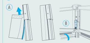
Position the wall so that the Velcro strip on the top faces the outside of the tent. Insert the keders into the frame (A) (INSERT MID FRAME) and attach the Velcro to the roof strip (B) (Inner side).
