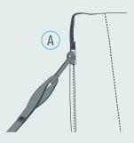
Attach the carabiners to the anchor points on each corner of the tent (A). Place the stakes at a minimum distance of 3ft.
