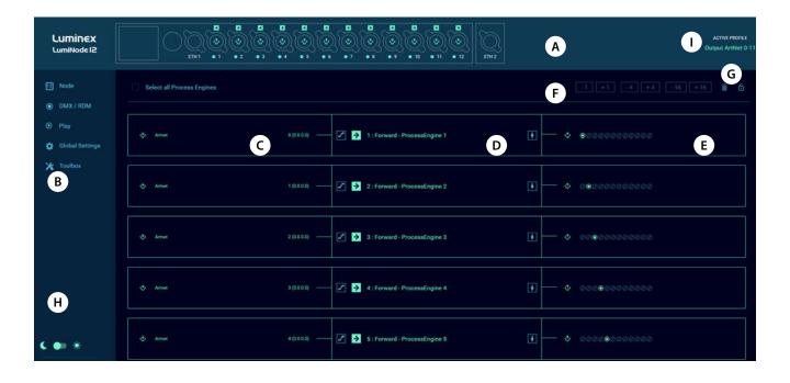
(A) Image of your LumiNode: Depending on the model you are using; the image might differ from the one displayed above. This product image shows the configuration of each DMX port. The center icon within each DMX port represents an input or an output. On the top of each port, you can see the mode of the Process engine linked to that port.
