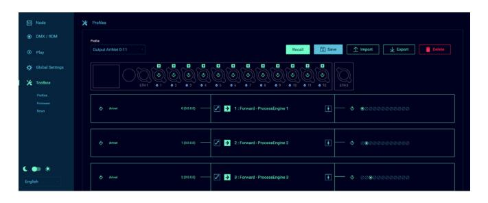
When a profile has been selected the user can scroll down to the bottom of the profile preview to see the IP settings in this profile. By default, the LumiNode will NOT load the IP settings that are stored in the profile. If you want to load the IP settings saved in the profile you simply slide the "Preserve IP settings" to OFF
