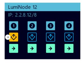
In order to clear to warnings, scroll to the following display and press the jog wheel. This screen can be found when scrolling left once when ports 1-4 are shown or to scroll all the way to past the last detailed port info.
