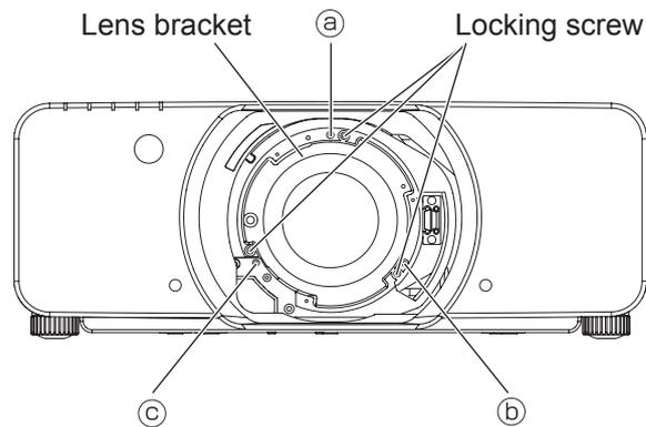
(Adjust the focus adjustment screws (a), (b) and (c) after installing the lens.)
