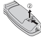
Insert the batteries according to the polarity diagram indicated inside. (insert the
