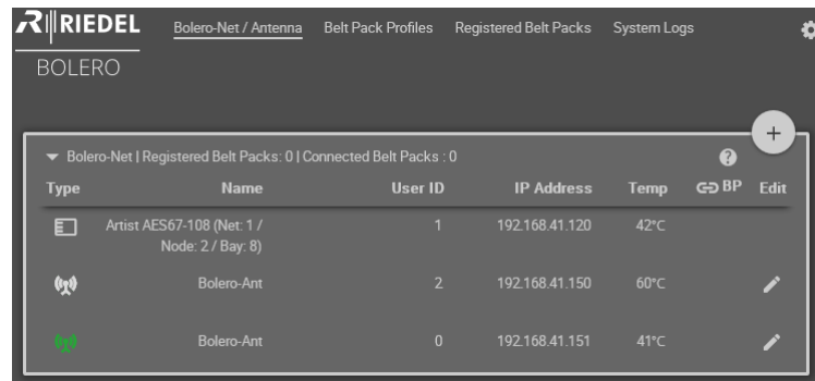
Figure 75: Added new Antenna in the Bolero-Net
