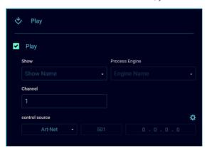
Select the control channel you want to use to control the cue list. Use the cog wheel to set the source protocol and universe and if required a specific controller IP.
