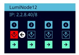
If the lost stream is recovered the LCD display will show this by changing the Output orange.
