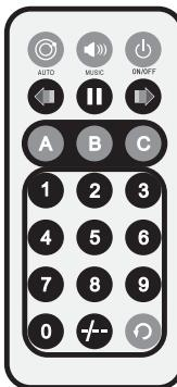
Point the infrared remote control directly at the infrared sensor installed on the front of the spotlight. The maximum range is about 8 metres. In the DMX and slave modes, the functions on the remote control are disabled.
