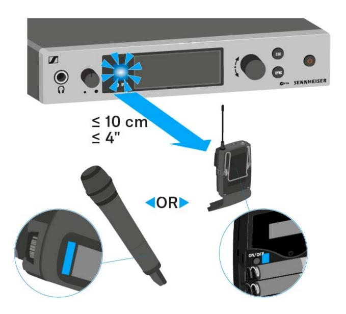
The parameters are transferred to the transmitter. The blue LED blinks during transmission.
