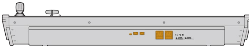
ATEM 2 M/E Broadcast Panel rear connectors
