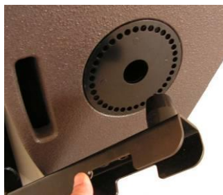
(7) Rotate the pivoting arm into position – the pivoting arm locking pin automatically secures the U-bracket
