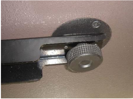
(7) Rotate the SB15P to the desired angle and secure using the tilt adjustment knob (pivoting arm locking pin automatically secures the U-bracket as the adjustment knob is tightened)
