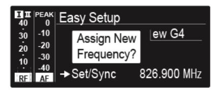
▶ Press the jog dial (SET) on the particular receiver to save your selected frequency and synchronize it with the corresponding transmitter at a later point (see "Synchronizing devices").
