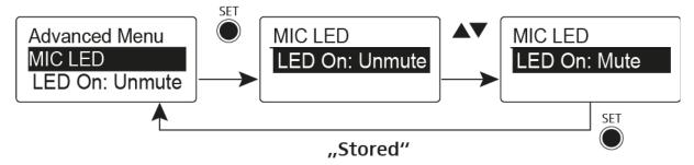
In the **MIC LED** menu item you can configure and deactivate the **STATUS** LED (see "Connecting the RMS 1 mute switch to the SK 300") of the RMS 1 remote mute switch regardless of the settings of the "Advanced > Mute Mode menu item" and the status of the RF signal.
