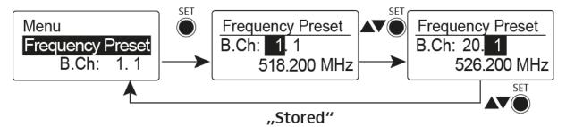
While you work in the **Frequency Preset** menu, the RF signal is deactivated.
