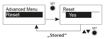
When you reset the bodypack transmitter, only the selected settings of the pilot tone and the **U1** to **U6** frequency banks are retained.
