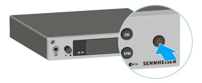
To switch the receiver to standby mode:
