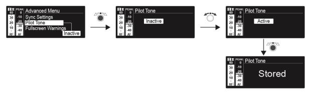
The pilot tone has an inaudible frequency that is sent from the transmitter and evaluated by the receiver. It supports the receiver's squelch function.
